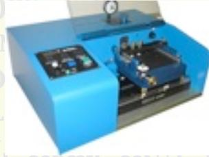
**de-lidder™** machines remove lids from hermetic packages non-destructively, leaving a particle-free cavity and reseal-ready surface so product can be reworked and resealed. We have multipurpose and dedicated models for rectangular, round, and optical fiber modules.
