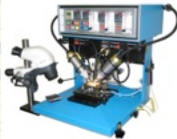
**HGRS *HOT* Gas Workstations** safely remove components from assembled circuits with momentary jets of precisely localized very hot Nitrogen. A full suite of tools also make these machines the ideal “thermal workbench” for prototypes & advanced applications.
