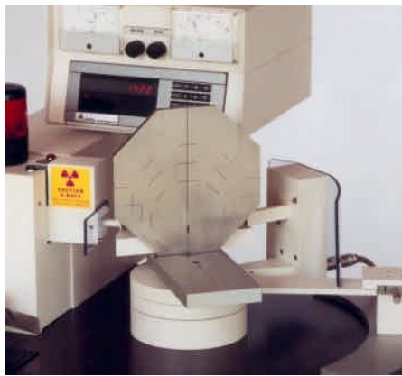
Stainless steel vacuum holder for wafer face orientation measurement. Engraving for accurate positioning of the wafer flat or notch. Models for wafers up to \varnothing 300 mm.
