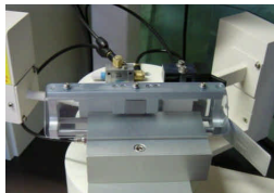
Holder for wafer flat orientation measurement. To use with with vertical window holder.
